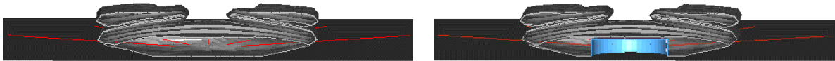
Figure 9: Folded bag without any components and with inflator housing outline. The flow direction at the points of inflator definition is marked by the red lines.
